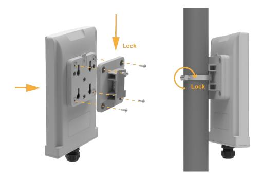
Bracket Wall Mounting Option (3M Tape or Screw)
